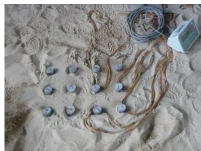
图 3 已压入的模型桩 Fig.3 Model piles pressed into soil
